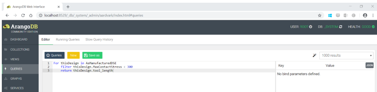
Figure 35: As Manufactured DSE – Query list of feasible tool lengths parameters
