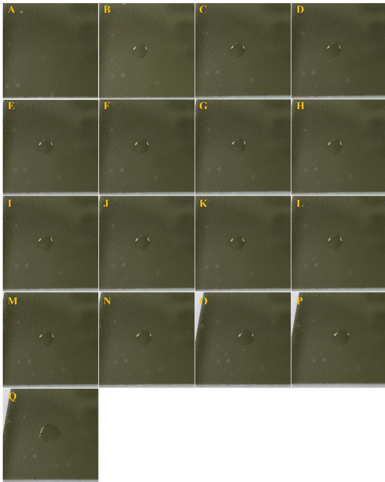
Fig. E1 — DFP on INVESIL coating. Images of a coupon before application (A) and at 0 (B), 0.5 (C), 1 (D), 1.5 (E), 2 (F), 2.5 (G), 3 (H), 3.5 (I), 4 (J), 4.5 (K), 5 (L), 10 (M), 15 (N), 20 (O), 25 (P), and 30 (Q) min following application of the target. These images were collected with a glass cover in place to limit evaporation. Reflections from the cover can be seen in some images.
