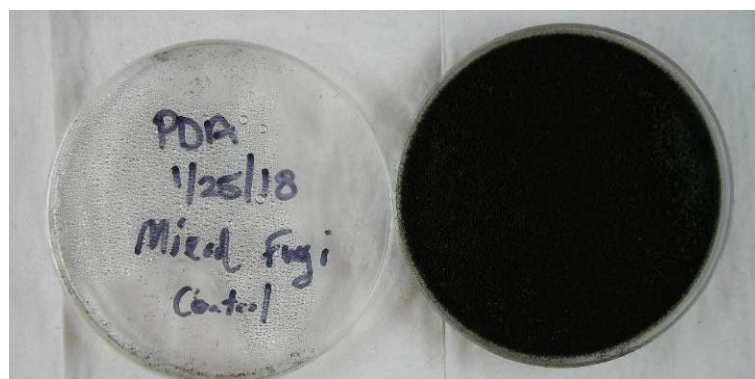
Figure 3. Potato dextrose agar 7 days after inoculation with mixed, five-specie fungal spore suspension. Growth on PDA confirmed fungal spores were delivered to coupons surfaces.
