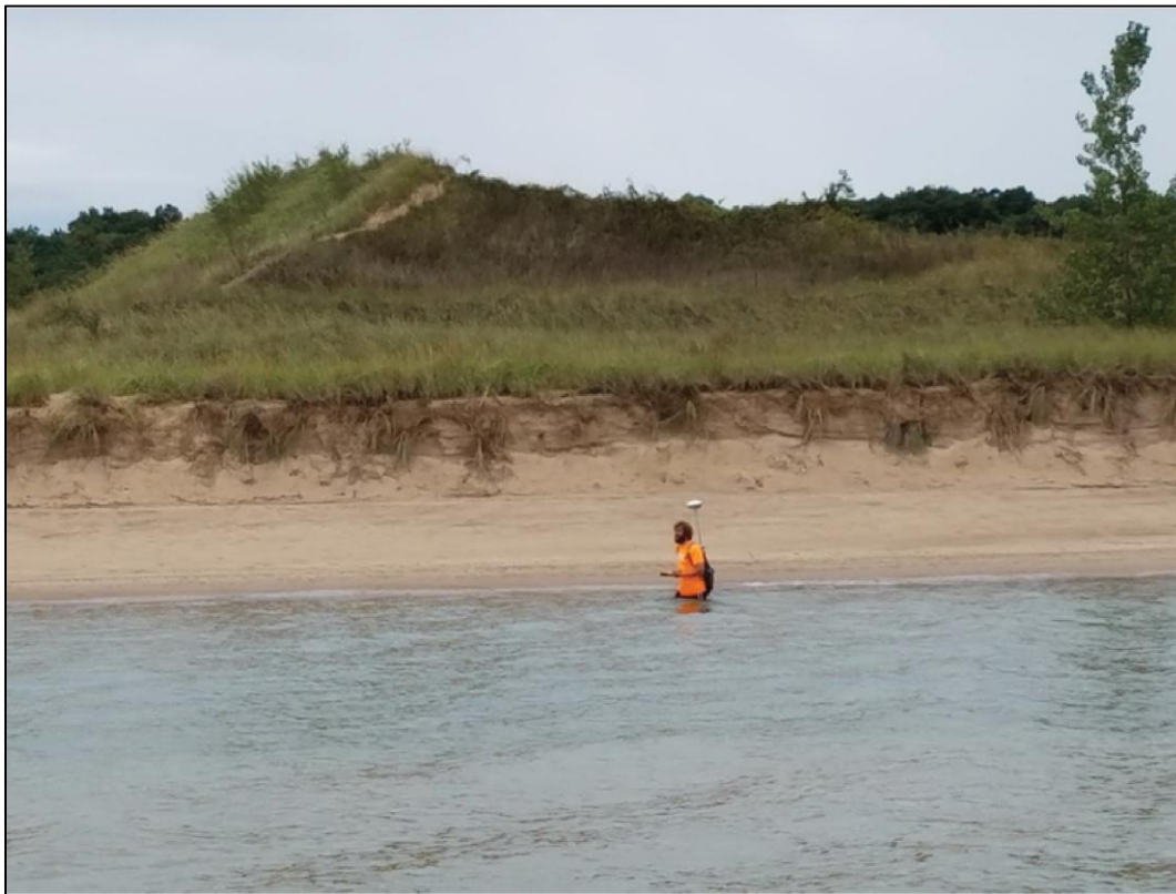
Figure 12. Sub-aerial beach and shallow water bathymetry surveys with the backpack-mounted Trimble Ag132 GPS.
