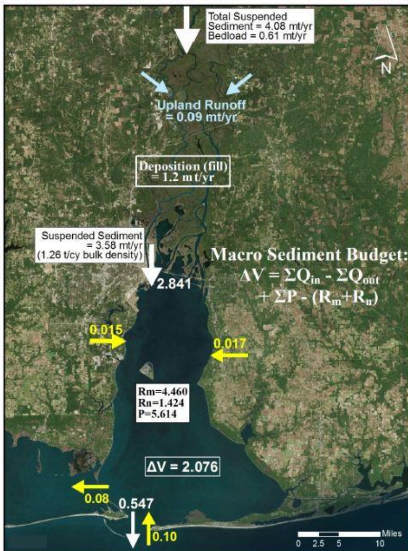
Figure 3. A macro-scale sediment budget for Mobile Bay showing transport pathways and magnitudes in millions of cubic yards.
