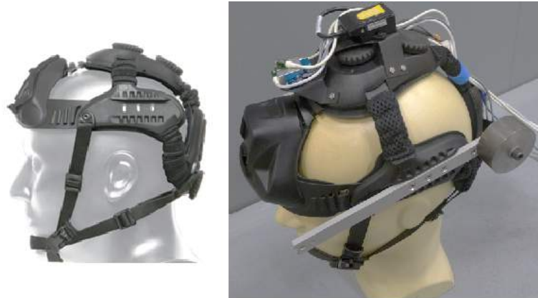
Figure 5-20: Skull Mounting System (left). HMSD configured with example rearward mass (right).
