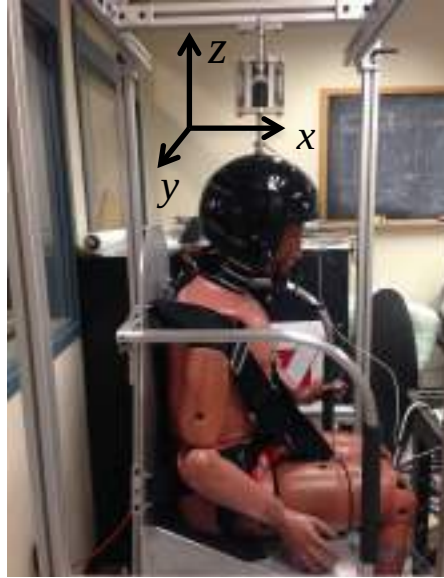
Figure 2-15: lateral view of the dummy in spine cyclic loading system and its Cartesian coordinates system.
