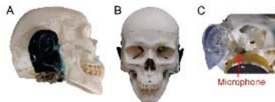
Figure 1. Acoustic test fixture (ATF). The ATF as pictured from the profile view (A) and from the front (B). In this image, the eye sockets have not been filled with the tissue simulant and the sensor is held in place with glue. A previous version of the sensed ear (C) shows the location of the microphone in the ear canal.
