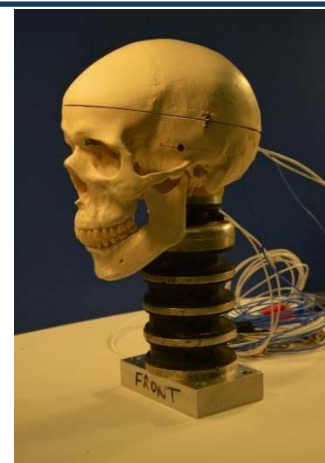
Figure: Instrumented surrogate head (L) and close up of surrogate head showing pressure sensors (red circles) on skull (R).
