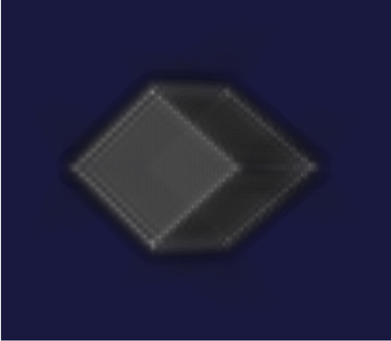
Figure 2. Volumetric CSAS image of a rigid cube based on synthetic data where the back-scattering scattering data was synthesized using the a Kirchhoff approximation approach documented in V. Bollen's 2017 Ph. D. Thesis. The image is shown here only for one perspectives, though images for other perspectives can also be constructed.
