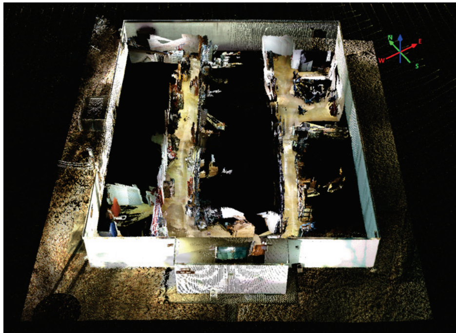
Figure 15. Collected point cloud overlaid with Leica C10.
