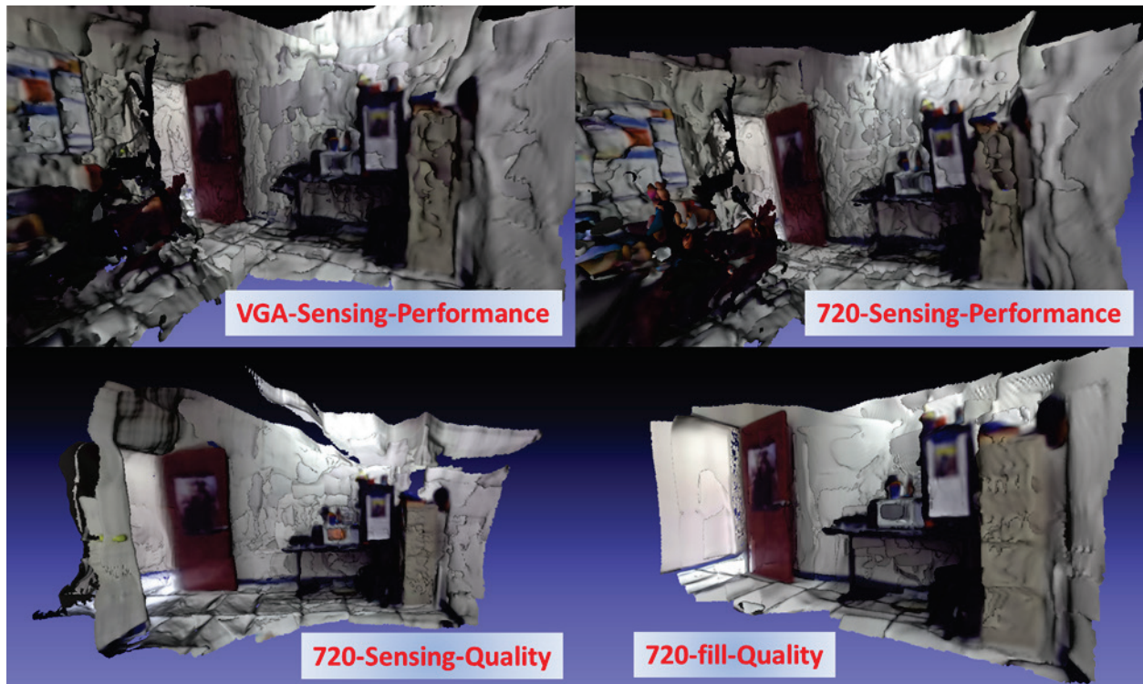
Figure 3. Point clouds generated from ZED photogrammetry sensor.
