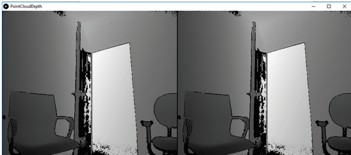
Figure 4. Depth image generated from Kinect Xbox One.
