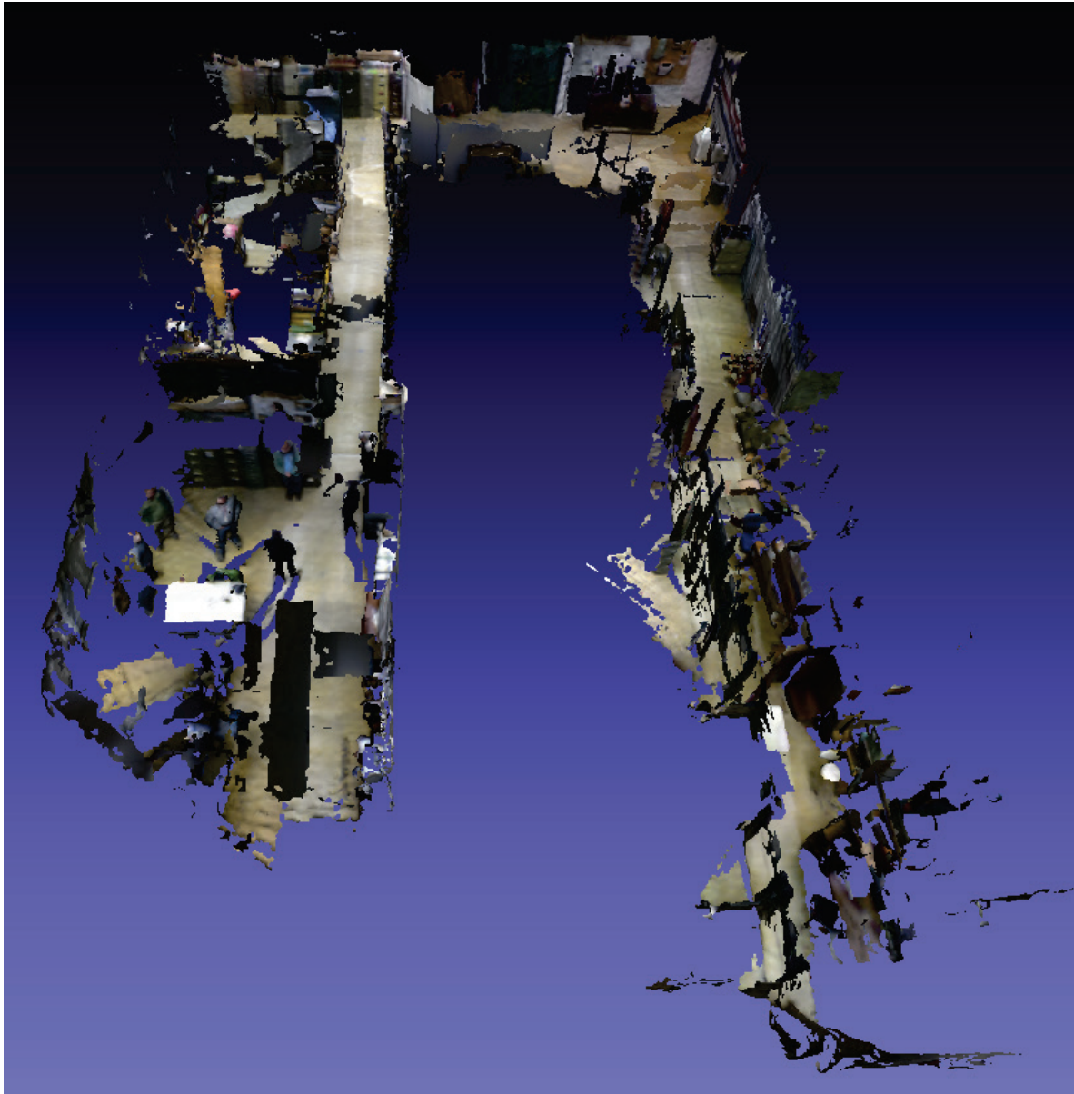
Figure 8. RGB point cloud collected using the RealSense D435.
