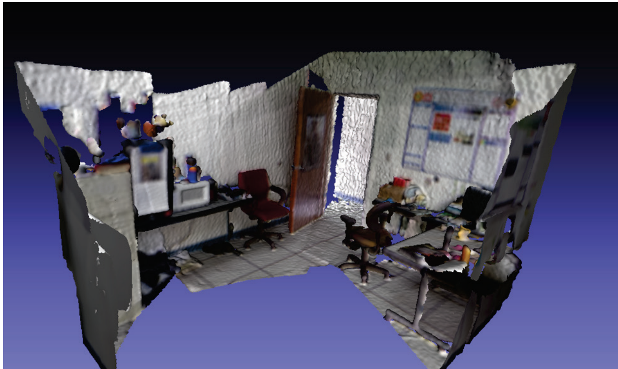
Figure 7. RGB point cloud collected with and Orbbec Astra.
