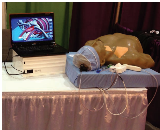
Figure 1. The mixed reality simulator of central venous access used in the study. The 3-dimensional visualization is displayed on the laptop screen.
