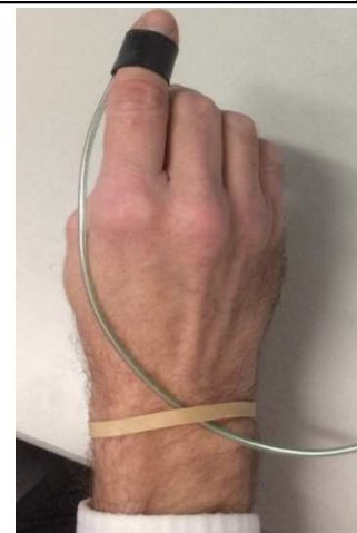
CTI simulator finger tracker, featuring an elastic “one size fits all” design attached to a user’s index finger.
