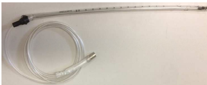
The chest tube tracker for the CTI simulator is inserted in the distal end of the chest tube and secured in the hub of the chest tube (left), while the armored sensor (right) detects the 6 DOF location of chest tube placement.
