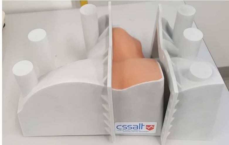
The newly redesigned ballistic gel physical mannequin mold for the SMARTS CVA simulator.
