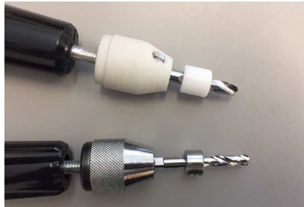
The new drill design with nonferrous materials (above), compared with old design (below).
