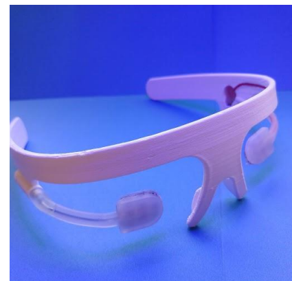
Figure 7. Goggles with new electrodes.
