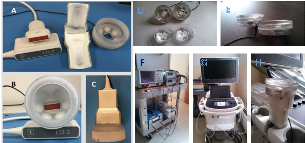
Figure 1. Image-guided intense focused ultrasound (ig-iFU) stimulation system. (A) Phillips EPIQ L12-3 imaging probe (left) next to its housing (center) and an iFU transducer (right) whose central aperture allows transmission of diagnostic ultrasound in a manner co-located with the iFU focus. Assembled proximal aspect of the ig-iFU device in (B) axial view and (C) side view. (D) iFU transducer with gel standoff to control depth of stimulation. (E) Side view of iFU transducer with gel standoff placed on the transducer. (F) Electronic setup for the iFU device including oscilloscope, function generators, amplifier and power regulator/surge protector. (G) Diagnostic ultrasound imaging machine with a completely assembled iFU transducer plus imaging probe. (H) A close up of the assembled probe for simultaneous ultrasound imaging and stimulation.
