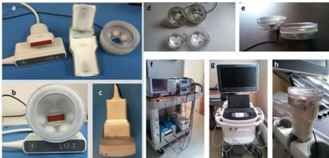
Fig. 1. Image-guided intense focused ultrasound (ig-iFU) stimulation system. (a) Phillips EPIQ L12-3 imaging probe (left) next to its housing (center) and an iFU transducer (right), whose central aperture allows transmission of diagnostic ultrasound in a manner co-located with the iFU focus. Assembled proximal aspect of the ig-iFU device in (b) axial view and (c) side view. (d) iFU transducer with gel standoff to control depth of stimulation. (e) Side view of iFU transducer with gel standoff placed on the transducer. (f) Electronic setup for the iFU device, including oscilloscope, function generator, amplifier and power regulator/surge protector. (g) Diagnostic ultrasound imaging machine with a completely assembled iFU transducer plus imaging probe. (h) A close up of the assembled probe for simultaneous ultrasound imaging and stimulation. iFU = intense focused ultrasound; ig-iFU = image-guided intense focused ultrasound.
