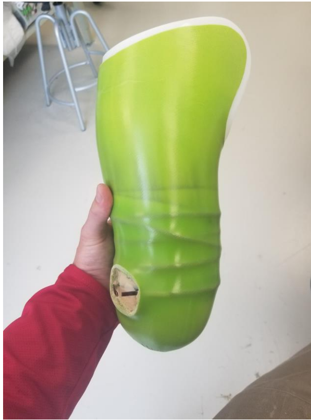
Figure 3: Socket sized for a large transhumeral amputee with an embedded powering coil.
