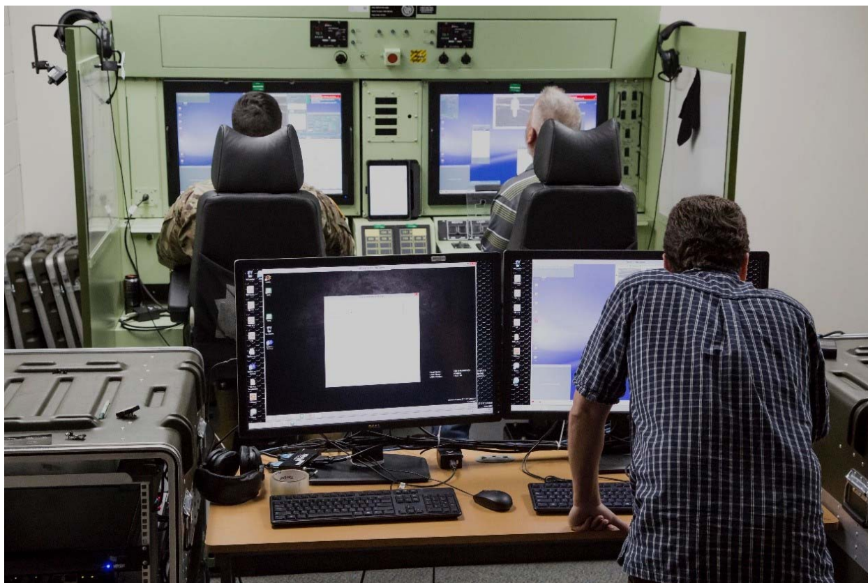
Figure 1. UMS laboratory at USAARL showing two person operator stations and mission control station in the foreground.
