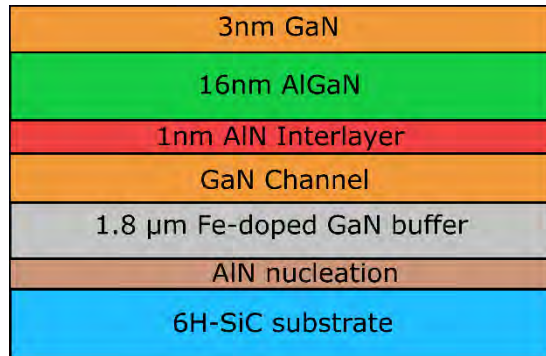
Figure 5.1: HEMT structure grown by MOCVD.
