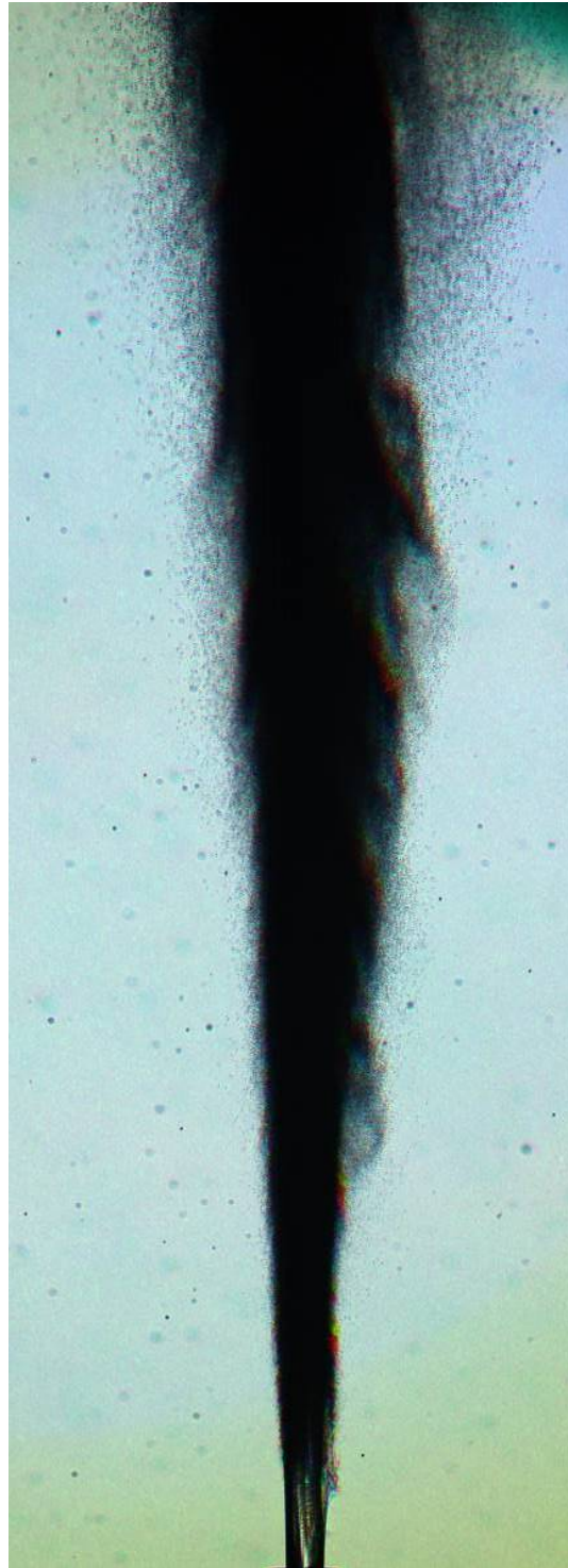
Figure 19: Sample full-frame (6000 px height, cropped width) image from Phase 2a Spectral Microscopy design. ECN Spray D, nozzle diameter of 180 \mu\text{m} , 500-bar fuel pressure, 6-bar ambient pressure, 1 ms after start-of-injection.
