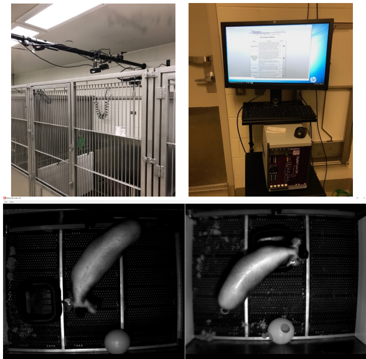
Fig. 5. Pig Epilepsy Monitoring Unit (EMU). Images above demonstrate the video acquisition using IR for 24 hour recordings/monitoring of the pigs (2 shown). Also depicted is the acquisition system for the wireless data, as well as the home cage with the IR illuminators, cameras, and wireless hubs.
