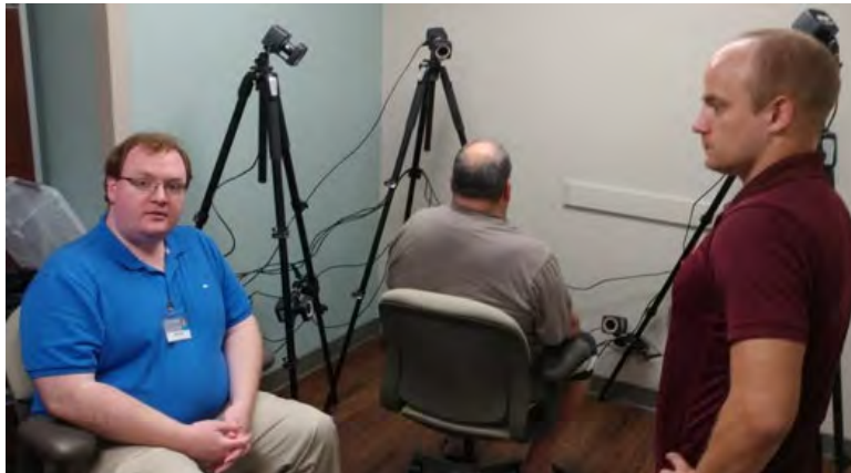
Figure 2 – Training the first subject on using the Vicon motion tracking system. Two graduate students (Kevin O'Neil – left, and Cody Barton – right) are shown working with the first subject (center) of the study. The Vicon motion tracking system was set up to work with the subject and track the detailed movements of his intact hand and the movement of his residual limb. This will allow the virtual prosthetic arm to be mapped onto and move with his residual arm in the virtual reality environment of the Oculus Rift goggles.
