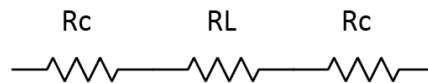
Figure 3 – Series circuit diagram where R_c presents contact resistors and R_L load resistors.
