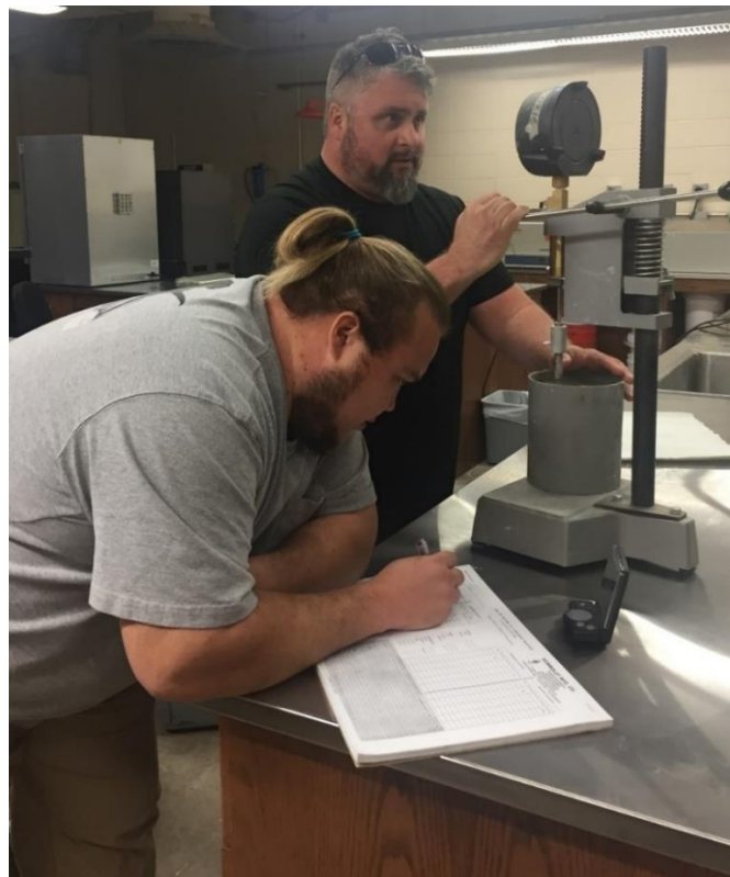
Figure 8. Set time demonstrated by penetrometer and Vicat methods.
