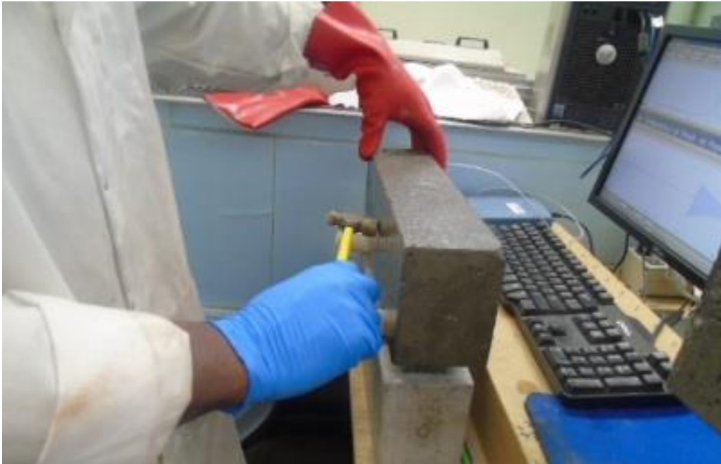
Figure 13. Freeze-thaw specimen undergoing testing for transverse frequency.
