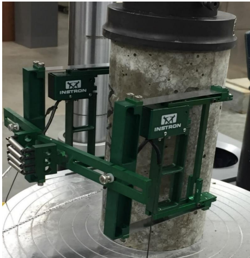
Figure 7. Concrete cylinder specimen undergoing modulus of elasticity test.
