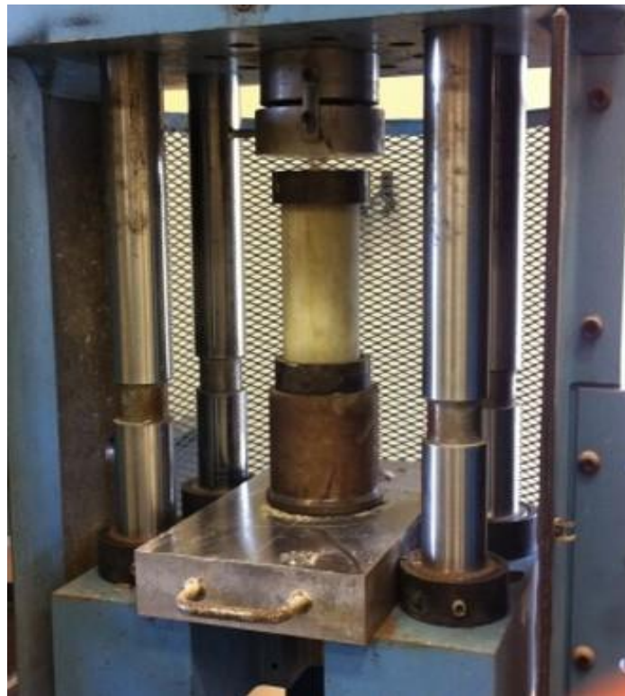
Figure 4. Concrete cylinder undergoing compression strength test.
