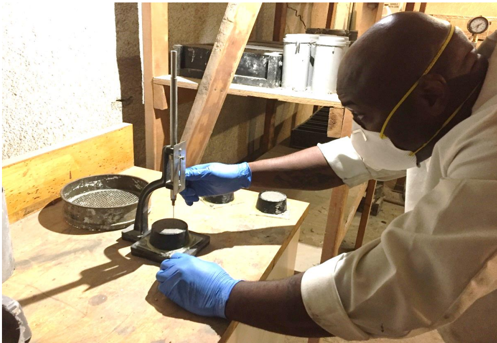
(b) Set time performed by the Vicat method, ASTM C191.
