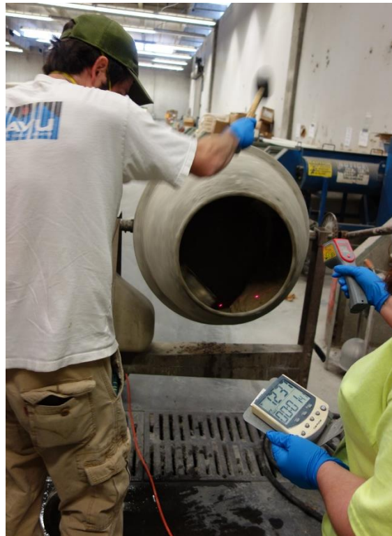
Figure 3. Laboratory mixing conducted by using small drum mixer.
