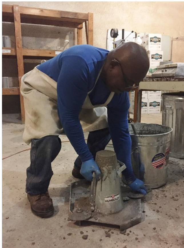
(a) Slump performed in accordance to ASTM C143.
