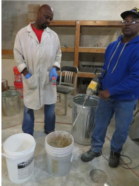
Figure 2. Laboratory mixing conducted by using Jiffy-type drill and paddle.
