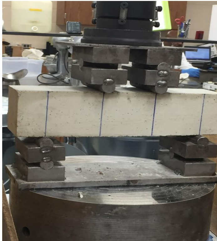
Figure 5. Concrete beam undergoing flexural strength test.
