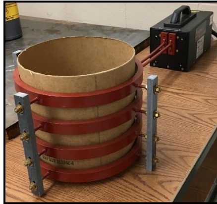
Figure 4.4. A 3 gal fiber drum inside the LIH coil.
