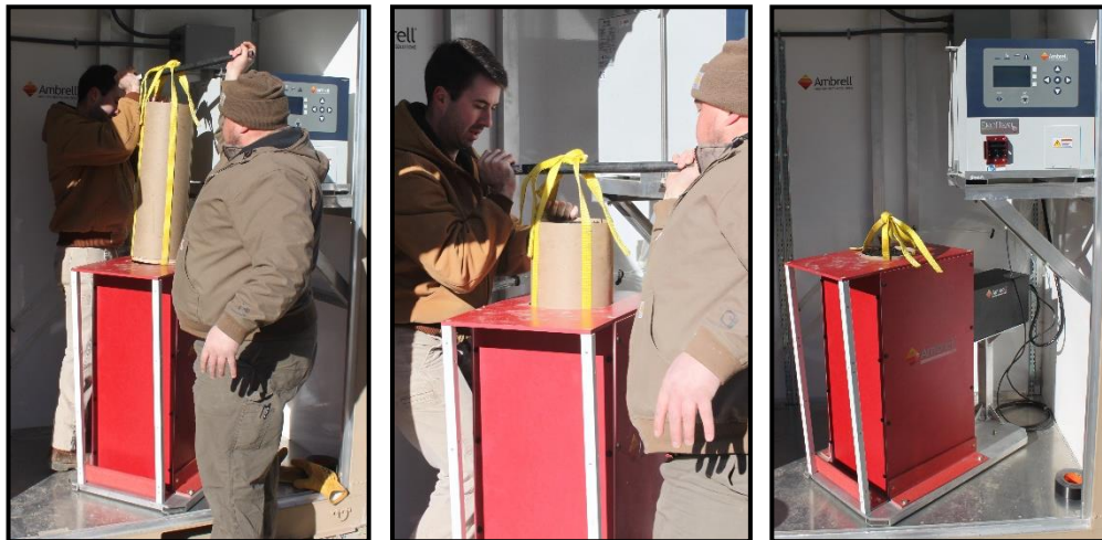
Figure 4.8. Placing 5 gal iHMA tube into FIH coil.
