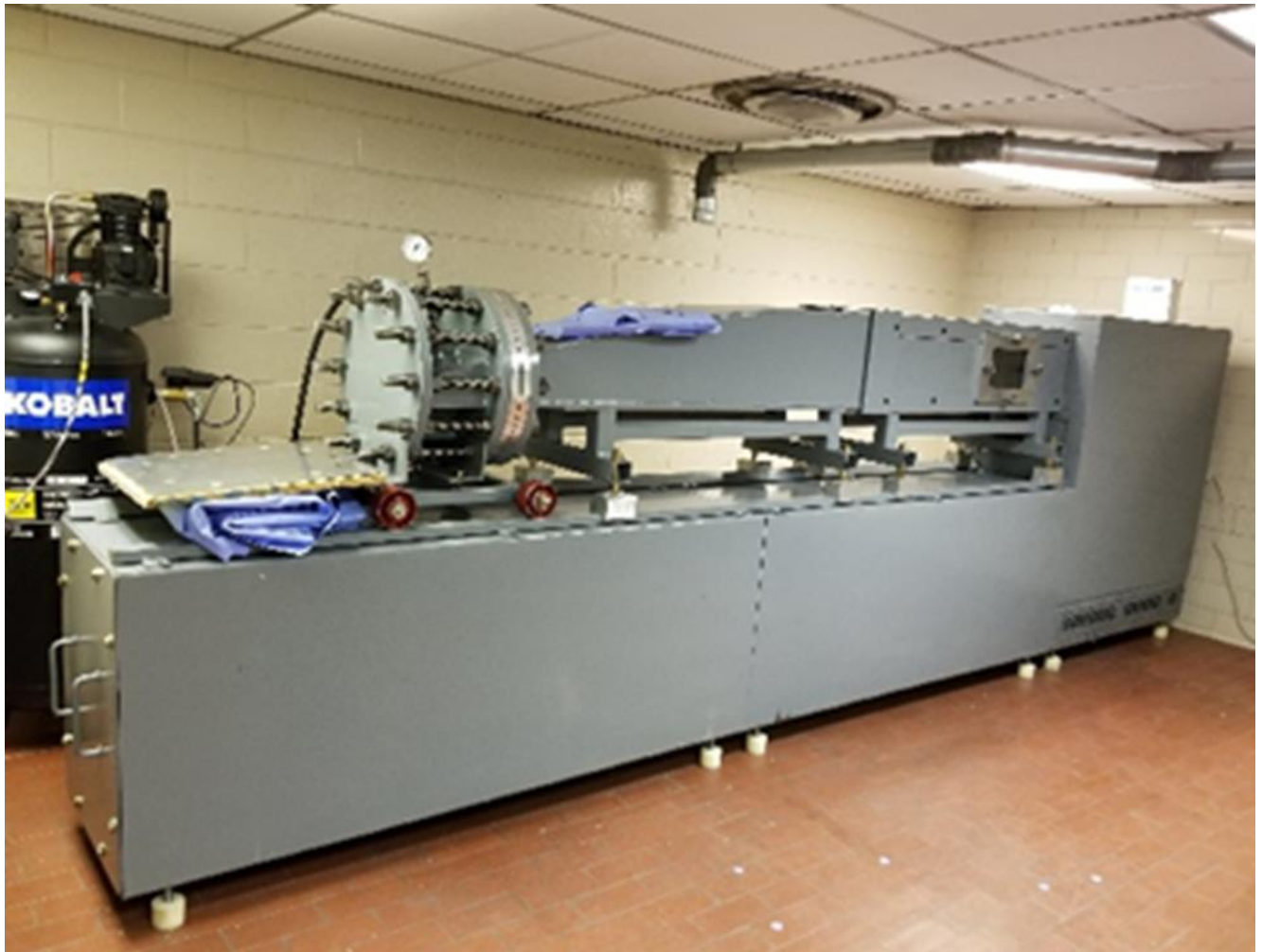
Figure 20. Shock tube manufactured by ORA Industries installed in our vivarium at National Jewish Health. The driving pressure to initiate rupture of the polypropylene-reinforced vinyl membrane is generated using compressed air (Kobalt air compressor). This system is able to achieve a driving pressure of 12-16 psi to rupture the membrane and create a shock wave that approximates IED blast exposures.
