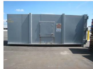
Compliant: RG container is closed.
