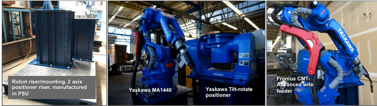
Figure 2. Robot riser unit and mounted Yaskawa MA1440 robot with Tilt rotate positioner, integrated with the Fronius CMT system, delivered to PSU PEPCO lab (1927 SE Water ave, Portland, OR 97214), which is a local laboratory site specialized in Additive manufacturing and macro-joining facility near PSU main campus. (Figure 3) The Material Research laboratory have three locations; Ondine lab for Metallography and mechanical testing, Advanced material and manufacturing research lab for thermal and reliability testing, and the PEPCO lab.
