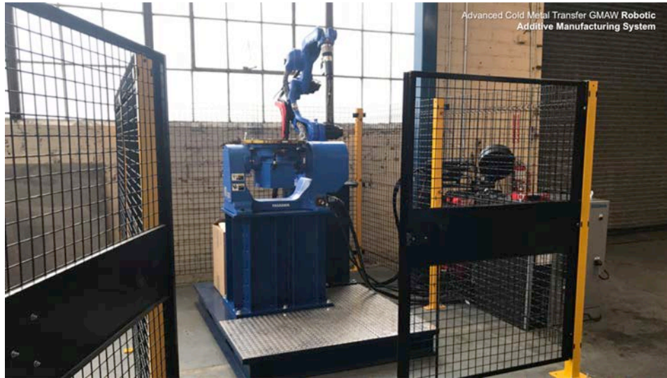
Figure 4. Safety fence and acquired system final configuration in PEPCO lab.
