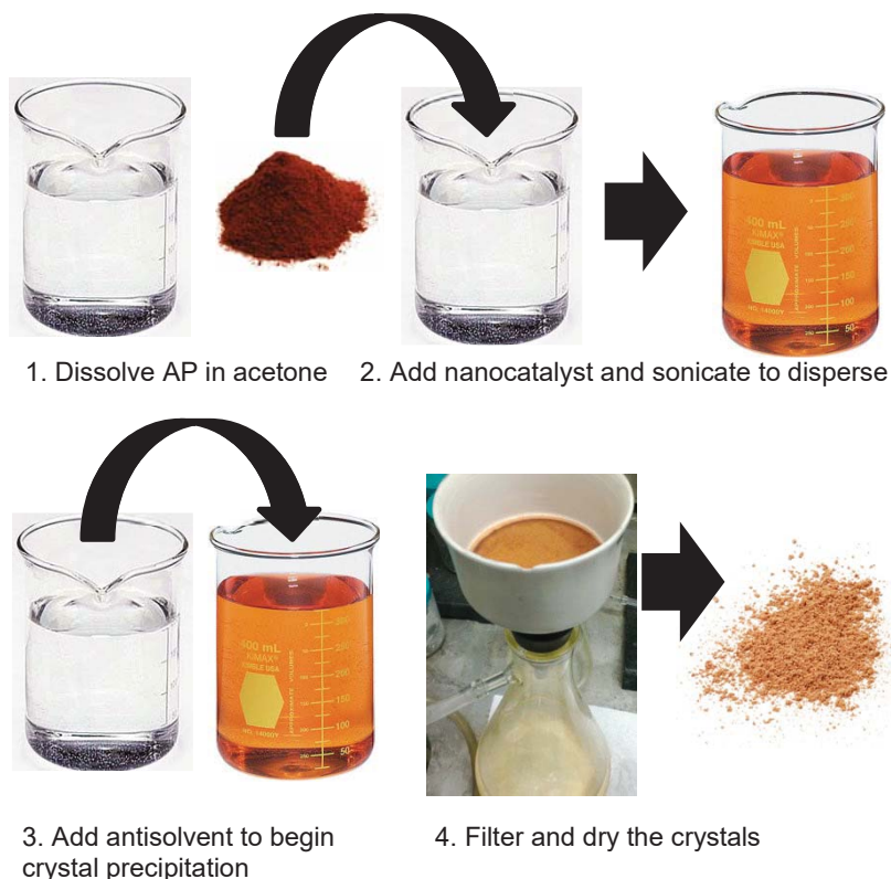
Figure 33: Schematic of process to encapsulate nanoscale particles into ammonium perchlorate.
