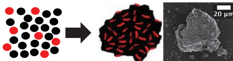
Figure 38: A schematic of the concept of producing a fuel particle with inclusions (left) where initial particles are milled to produce a micrometer scale particle with inclusions. An SEM image of an Al/PTFE particle is shown on the right.
