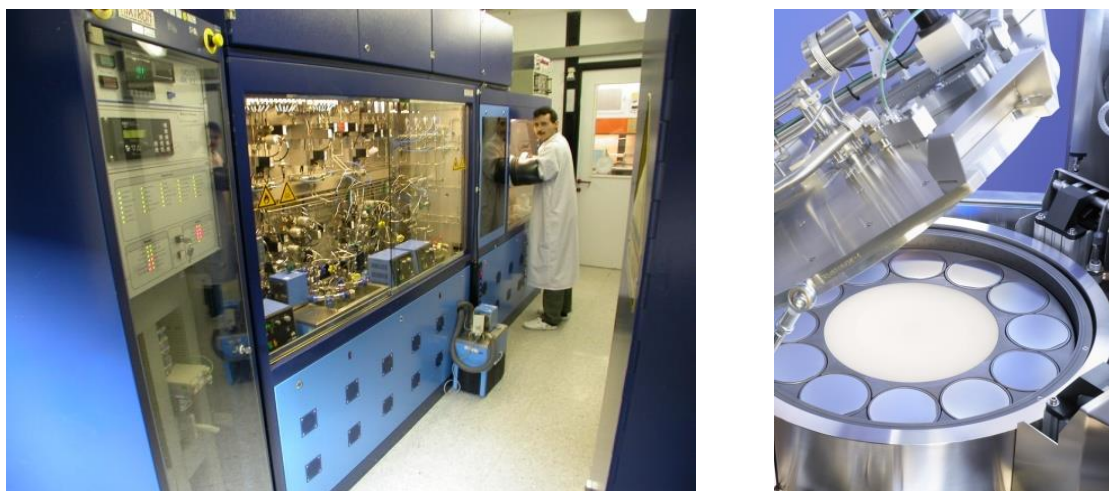
Figure 1. Available MOVPE reactors: R&D MOVPE-reactor tool for 2" substrate wafers ( Aixtron Aix 200-GFR-reactor ) (left) and MOVPE-production reactor tool ( Aixtron Aix2600-G3-reactor ) in a 12 * 4" wafer configuration (right).
