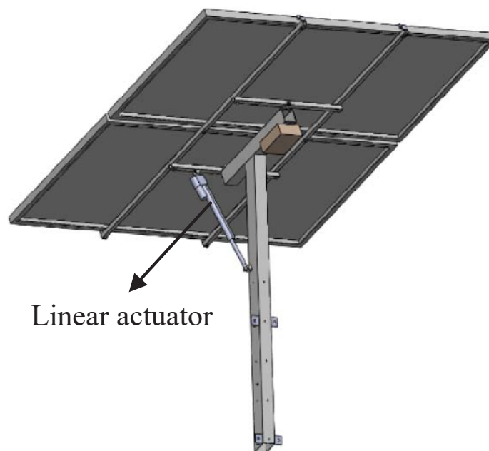
Figure 2.1. Single-axis of solar tracker
