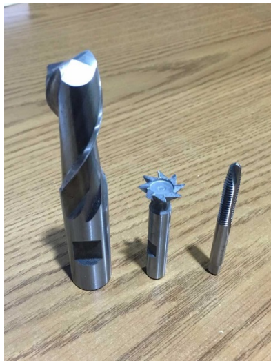
Figure 19: \frac{3}{4} inch Flat End Mill, \frac{3}{4} inch Dove Tail End Mill and \frac{1}{4} Regular Thread Tap
