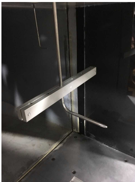
Figure 24: Pitot Probe Rake Holding a Probe
