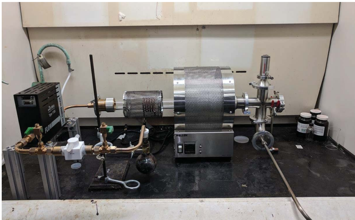
Figure 29: Material exposure experimental setup, without heaters.
