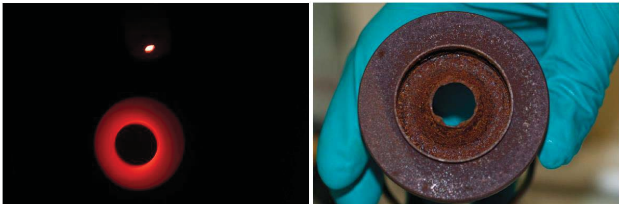
Figure 2: Busek 200W HET after Operating on Iodine: Left – Anode just after Shutdown (Glowing Hot), Right – Anode Extensively Corroded.
