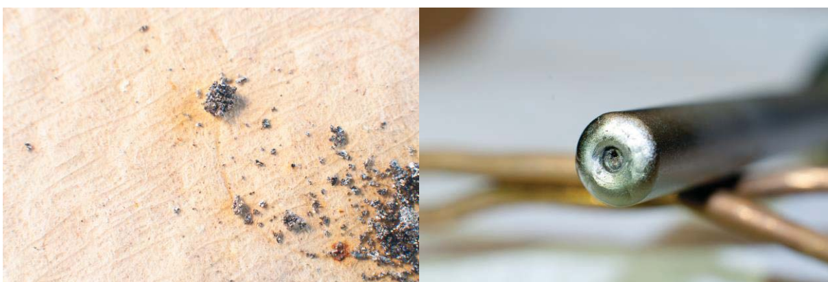
Figure 46: Material removed from clogged cathode orifice (left), clogged cathode orifice (right).
