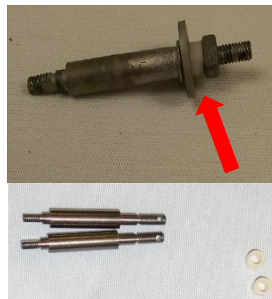
Fig. 1. Germanium buildup on the ceramic insulators of the heater power supply and the replacements.
