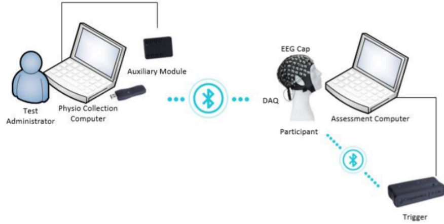
Figure 22. The architecture of collecting and recording physiological signals.
