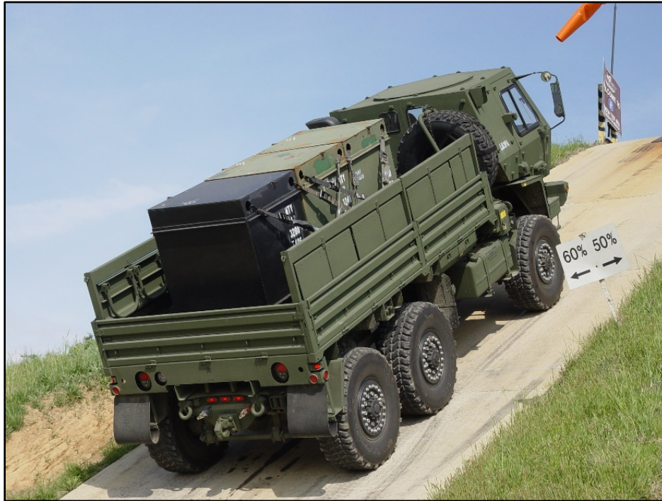
Figure 1. Vehicle on 60 percent Longitudinal Grade.
