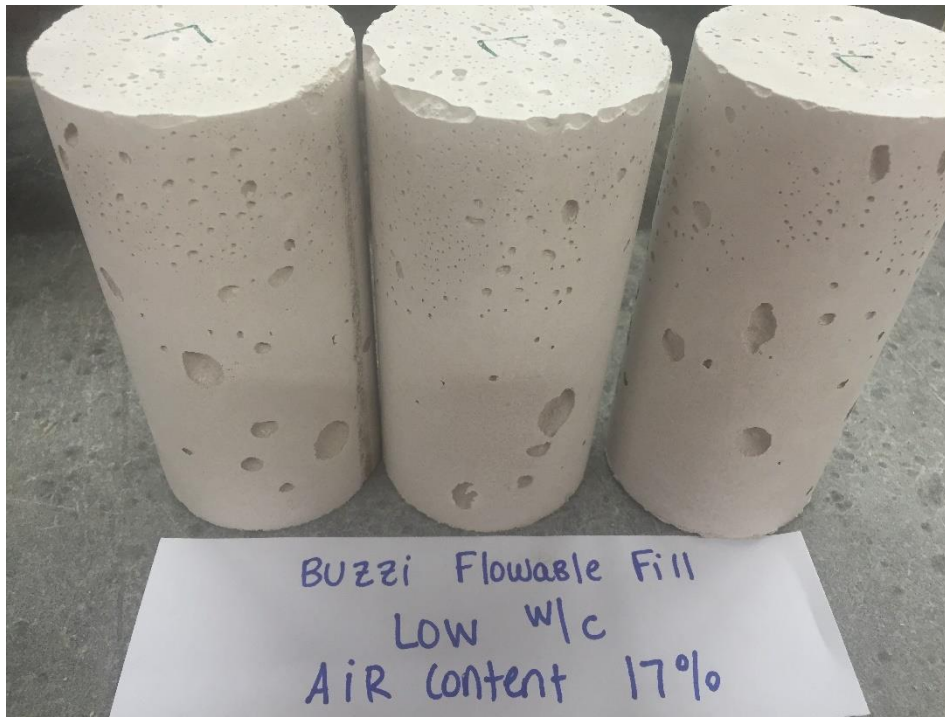
Figure 3. Low w/p ratio 3-in.-diam by 6-in.-high cylinders.
