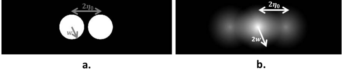
Figure 8: a. Pupil function with 2 circular apertures. Each aperture has a radius, w , and centers located \pm\eta_0 from the origin. b. Frequency response of the pupil when illuminated by a point source.
