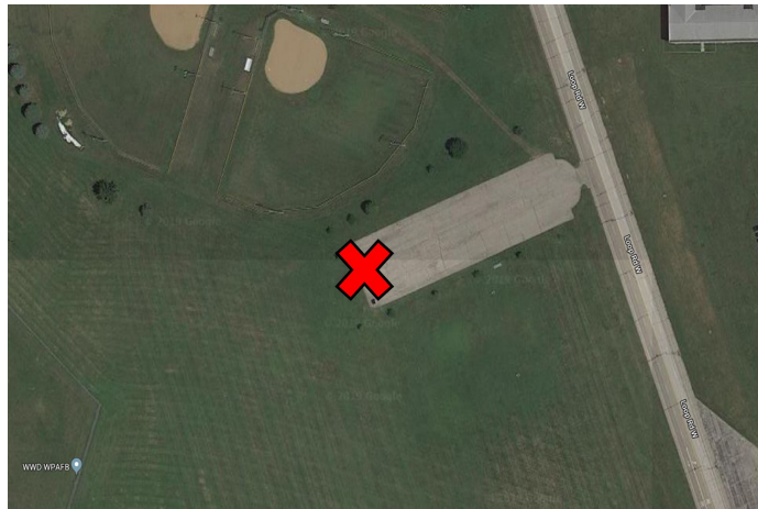
Figure 13: Location used to collect ‘clean’ GNSS signals. Here, there are minimal obstacles to interfere with live-sky signal propagation. (Satellite image supplied by [34]).
