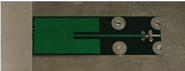
(c) Patch antenna on ground plane with aluminum plates on left-hand side
