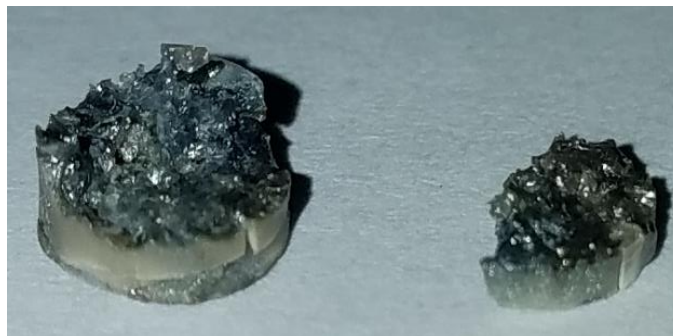
Figure 7: photograph of the undoped TiO 2 pellet after flash sintering.
