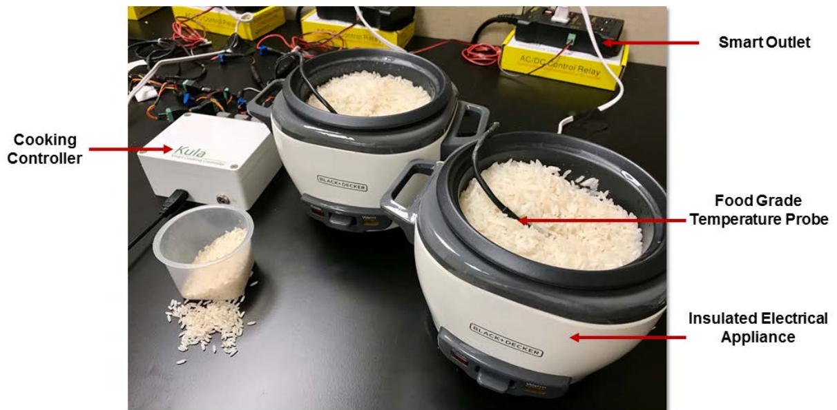
Figure 4 Rice cookers with temperature feedback control
