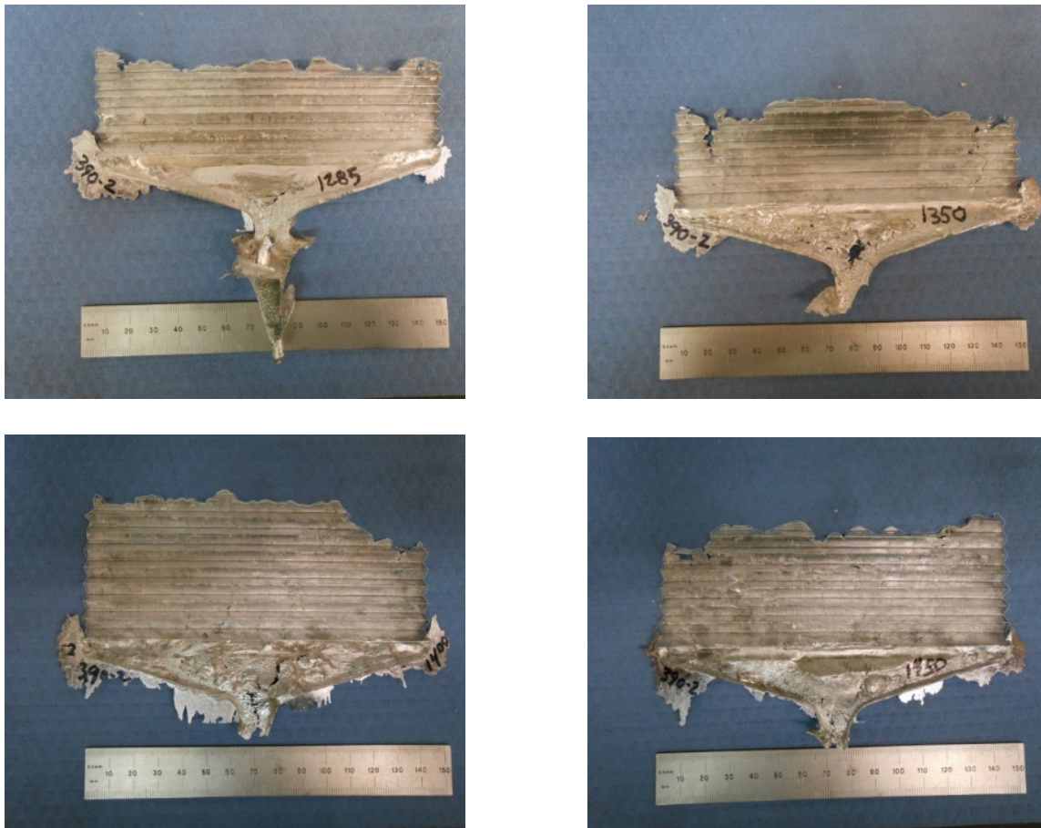
Figure 5.2.6: Thin foil 390-2 alloy film solidified in the vent block
