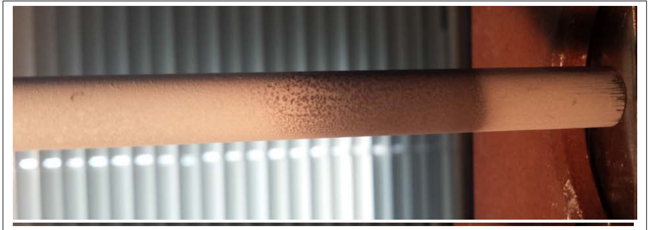
Figure 5.4.5: Smooth surface rod after first pull-out
