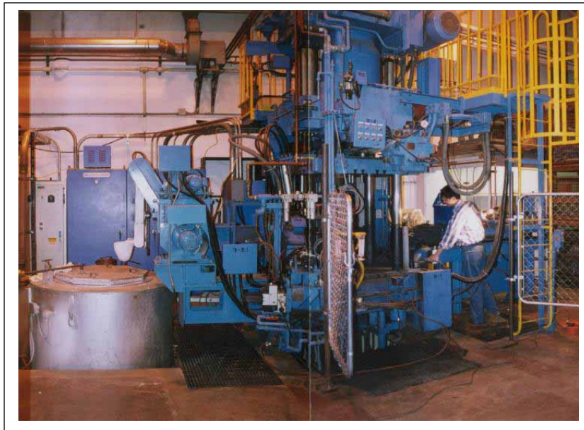
Figure 6.1: 350 ton Ube squeeze caster at Case Western Reserve University
