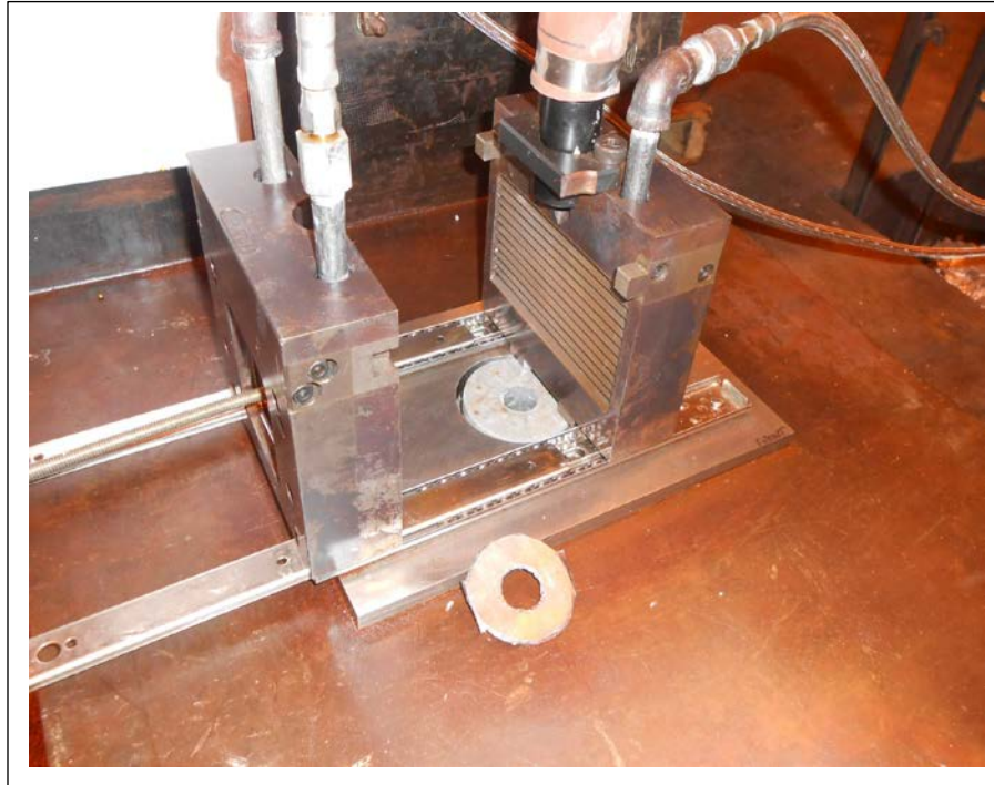
Figure 4.4: Open vent block mounted on rails; vacuum sealing gaskets
