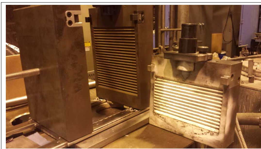
Figure 4.8: Installed large vent block side-by-side with old vent block
