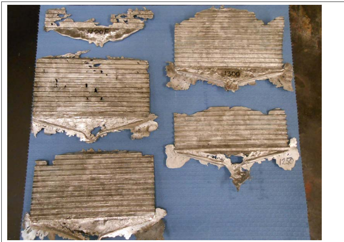
Figure 5.1.1: Thin foil of 356 alloy solidified in the vent block: the area of the foil increases as a function of temperature and provides a sensitive measure of fluidity
