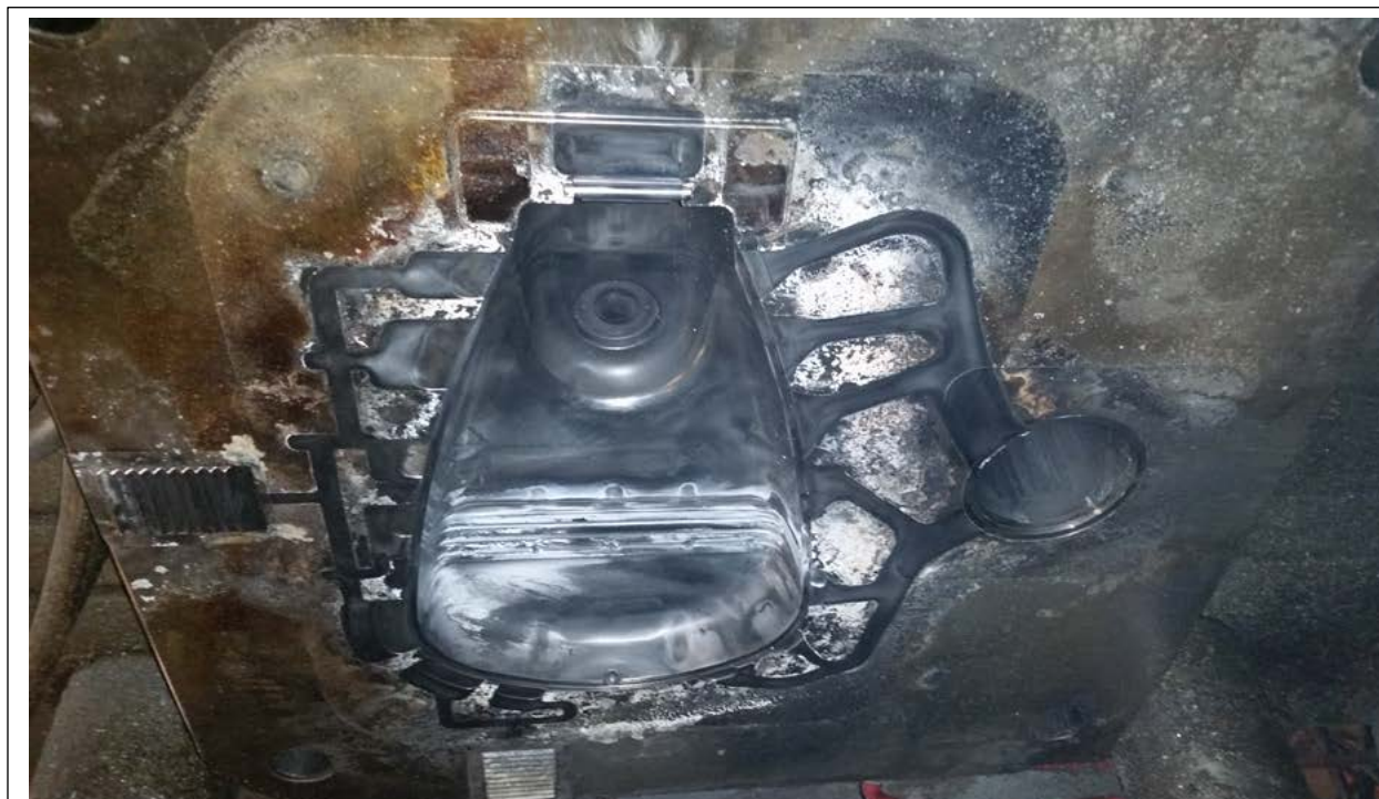
Figures 5.5.2 and 5.5.3: Lamp die used for making thin wall lamp head castings
