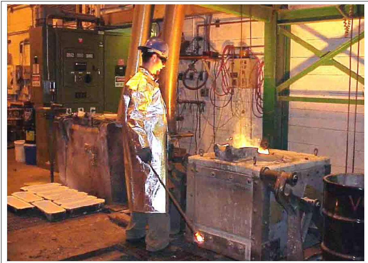
Figure 5.2.2: Induction melting system used for adding copper to 390
