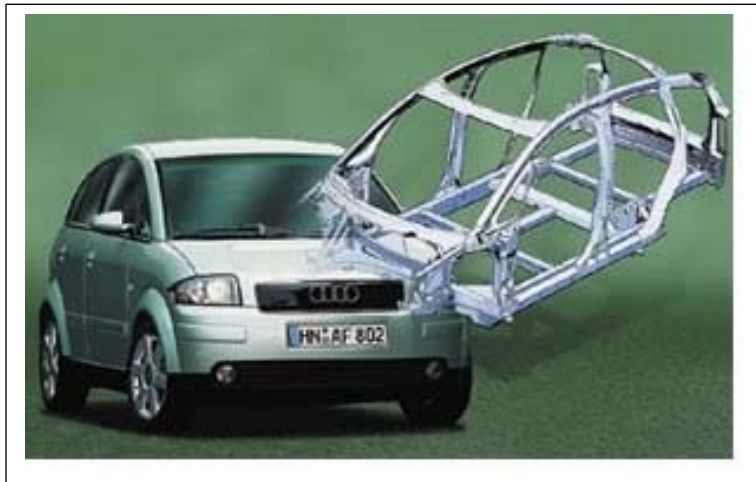
Figure 3.1.2: B-Pillar cast by the High-Q-Cast™ high vacuum process
