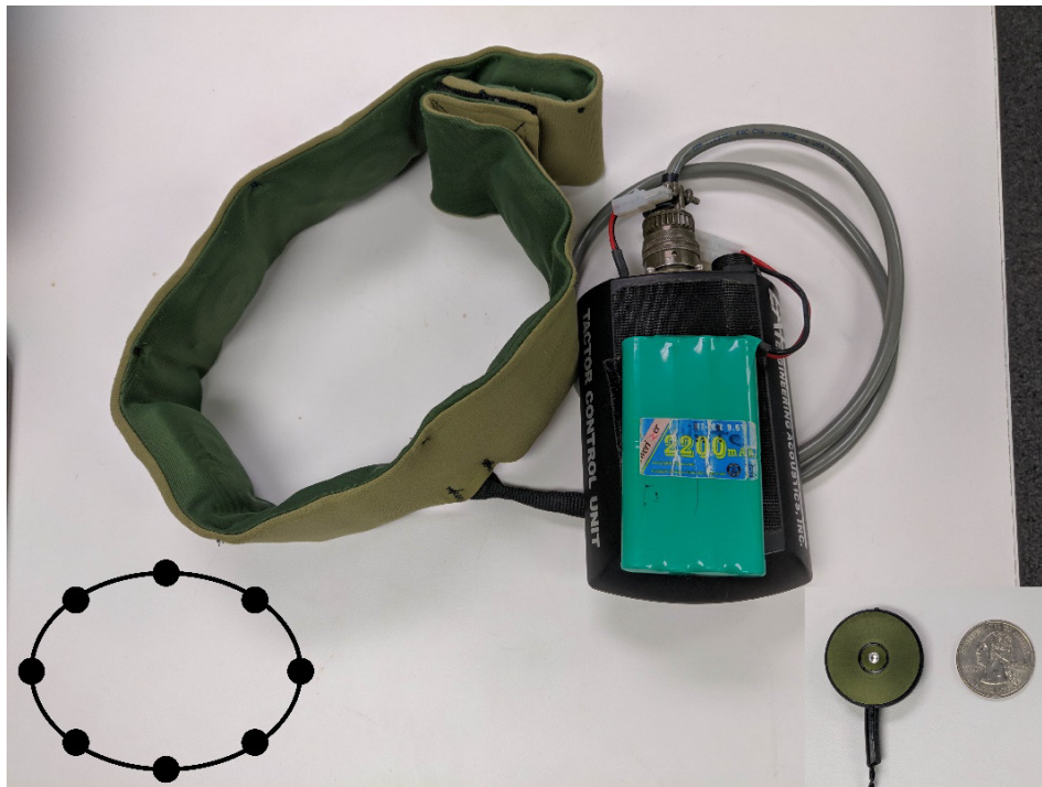
Fig. 4 Tactile belt and C2 factor (lower right hand panel) used in the experiment. A schematic depicting locations of the factors on the belt is shown in the lower left-hand panel.
