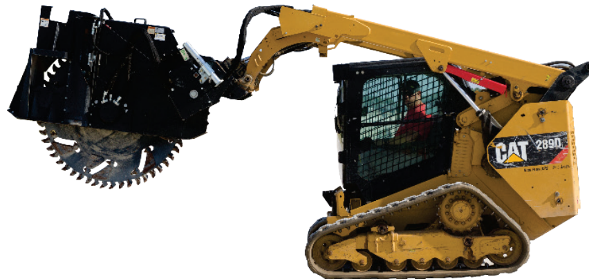
Figure 2. Caterpillar 279C CTL with SW45 wheel saw attachment.
