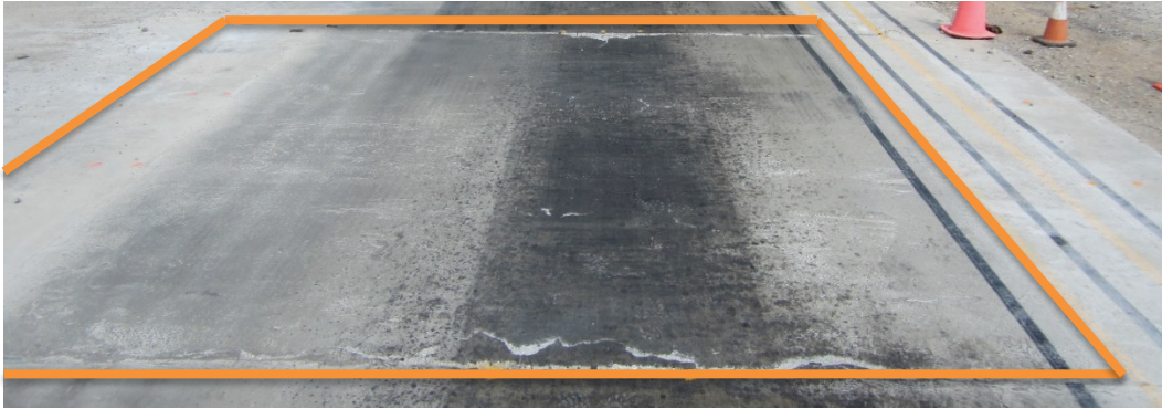
Figure 32. Repair 3, high-severity joint spalling on rear edge, 2,000 passes.
