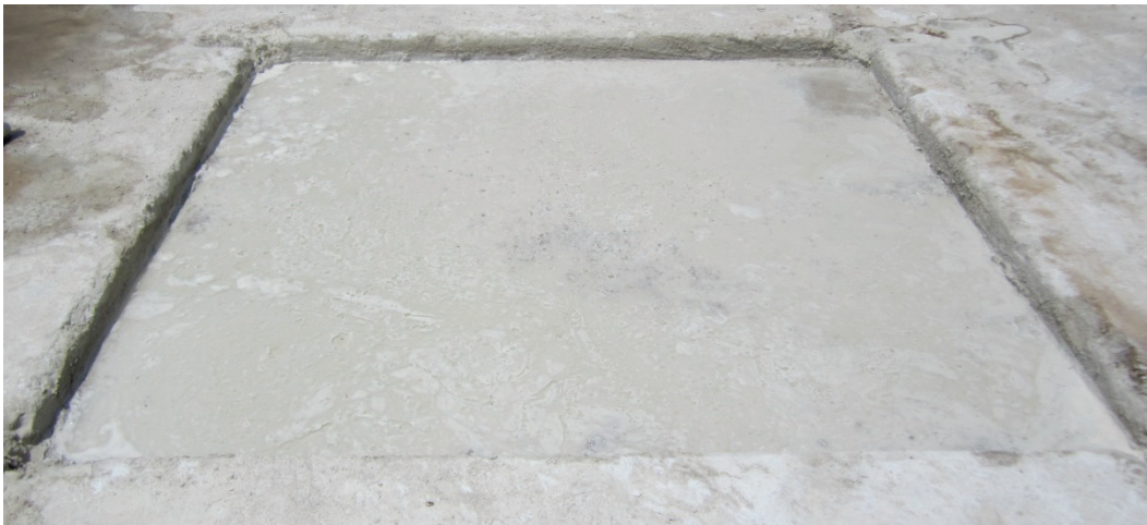
Figure 40. CTS rapid-setting flowable fill after 30 min cure time.
