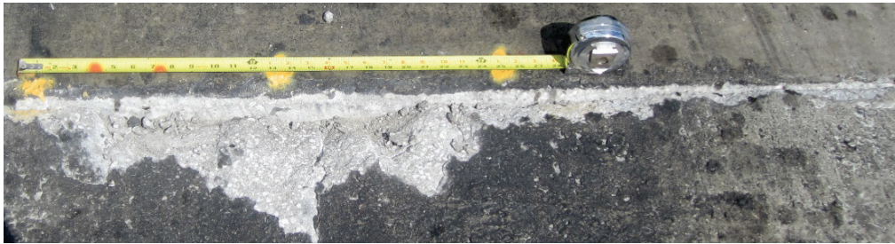
Figure 32. Repair 3, high-severity joint spalling on rear edge, 2,000 passes.
