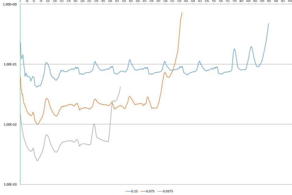
Figure 18: Maximum relative error of the field component E_y over the entire computational domain. Dependence of the interval of stable performance on the grid size.
