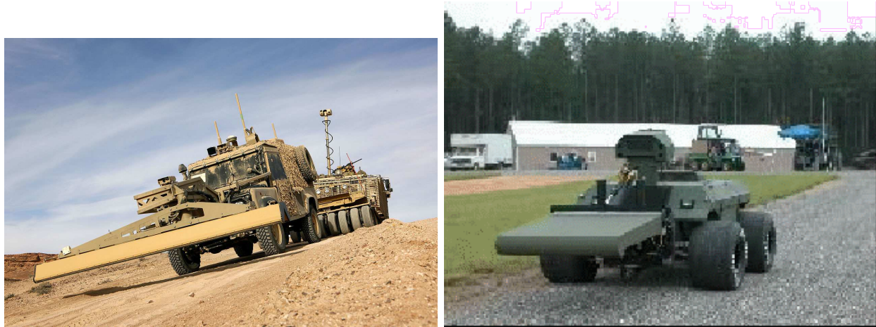
Figure 133: (a) Remote-control "Panama" Land Rover with ground-penetrating radar to detect IEDs followed by Mastiff with Choker mine rollers [144]; (b) Although a number of vehicle based GPR systems have been trialled and reported on over the last 5 years the most extensively reported system has been the NIITEK radar shown [140]
