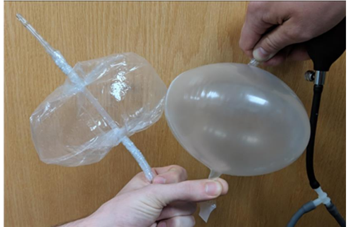
Fig. 1 Prototype comparison: hand-molded balloon (left) vs. Interplex manufactured balloon (right).
