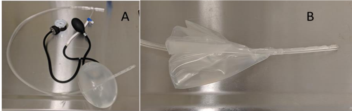
Fig. 3 Second round of Interplex Medical manufactured GROA device with soft balloon material and increased thickness (90A, 0.01" thick): (a) fully inflated device and (b) deflated device.
