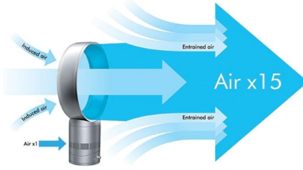
Figure 6. Illustration of Entrainment in Bladeless Fan [19]
