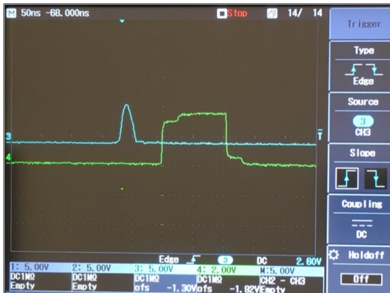
Figure 10. This oscilloscope reading shows the general characteristics of the timing pulse created by the laser diode (3, top) and camera readout signal (4, bottom). Jitter between the diode trigger pulse to the camera, and the camera monitoring pulse was measured to be less than 1 ns shot to shot.
