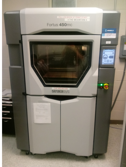
Figure 2.2. The FORTUS 450mc Printer used to create the test samples.
