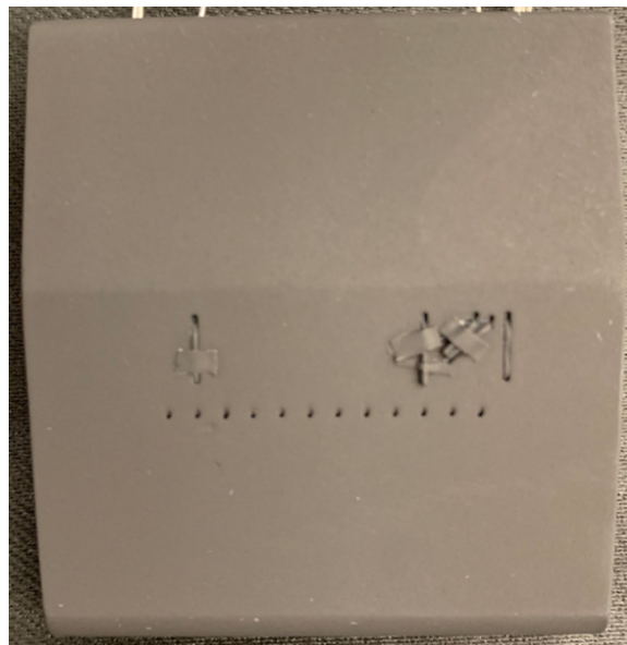
Figure 58. Airfoil with cylindrical holes after being painted and having the thermocouple installed.
