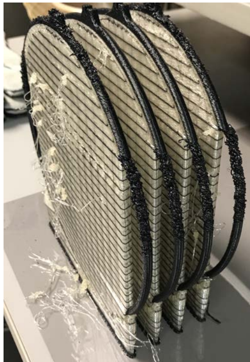
Figure 39. The side profile of a 90° print from the first trial.
