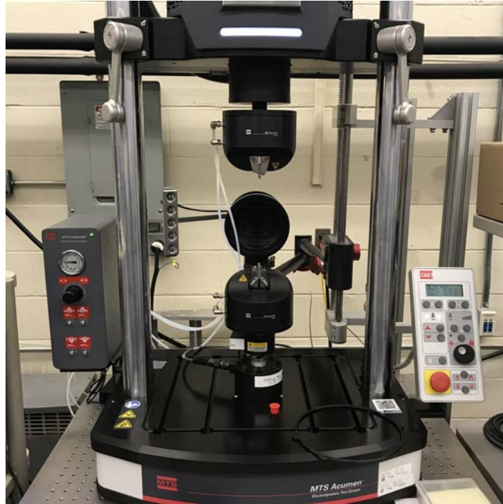
Figure 44. MTS Acumen 3 testing rig—located at AFIT and equipped with a 250 N load cell.
