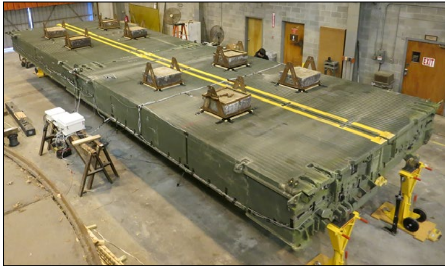
Figure 10. Representative photograph of two-bay test (test 2-2 shown). Each lead block weighs approximately 2,000 lb.
