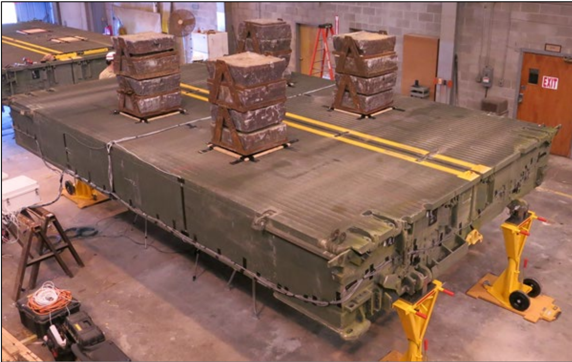
Figure 7. Representative photograph of one-bay test (test 1-2 shown). Each stack of lead blocks weighs 8,100 lbr.
