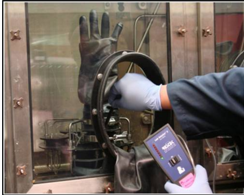
Figure 3. Helium leak check of glove, fittings, lines, and interfaces after securing base to glove fixture carousel.
