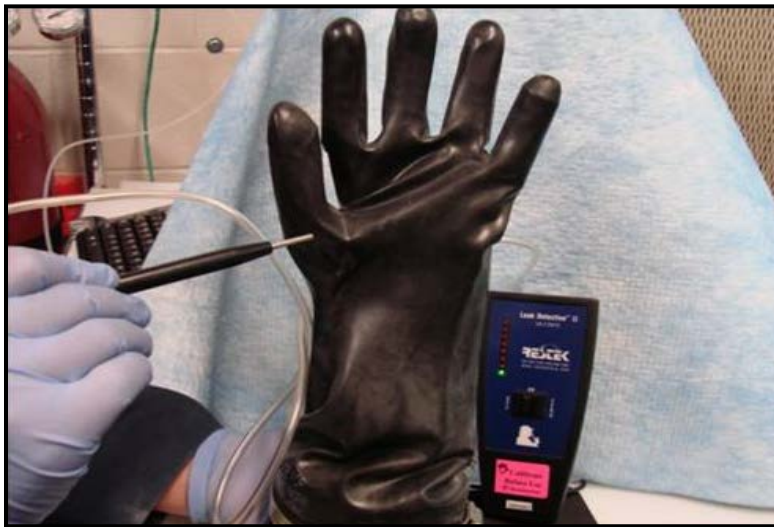
Figure 2. Helium leak check of glove before mounting on glove fixture carousel.
