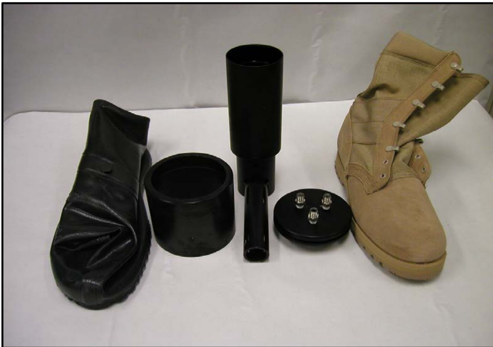
Figure A-2. Currently used boot form for chemical agent resistance testing of boot systems.
